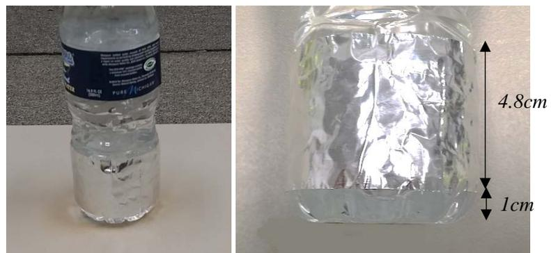
**Figure 5. Water bottle with aluminum foil tape**
