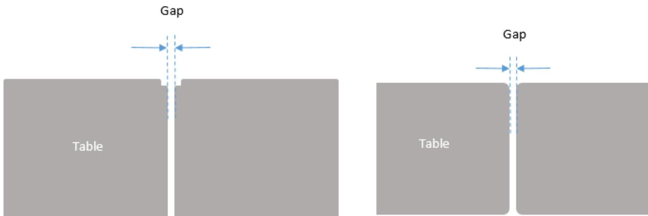
**Figure 3. Examples of table gap measurement**
